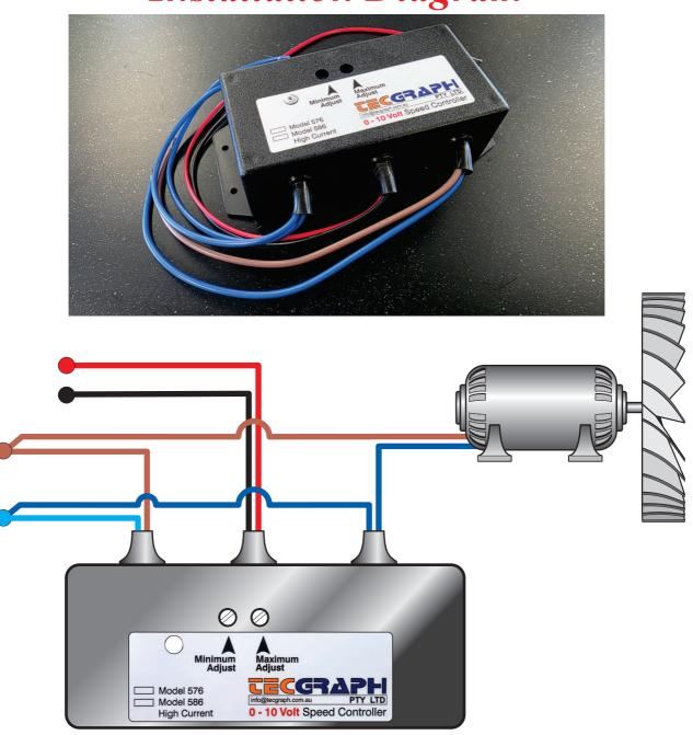
The 576 controller is an economical solution to the need for a remote 0 - 10 volt DC electrical control signal to control the speed of a fan. The fan will run at minimum speed with 0 volts DC control signal and will increase to the maximum setting at 10 volts DC control signal. The maximum speed can be set at the maximum motor speed or any lower value. The minimum speed can be set at any speed above motor stall speed which provides adequate cooling air to the motor.
